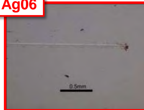
Mild wear of coating & tribofilm build-up → Optimized coating!
