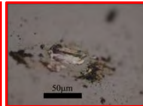
Mild wear of coating & tribofilm build-up → Optimized coating!
