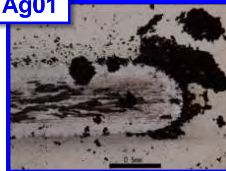
Large wear of the coating and the pin
